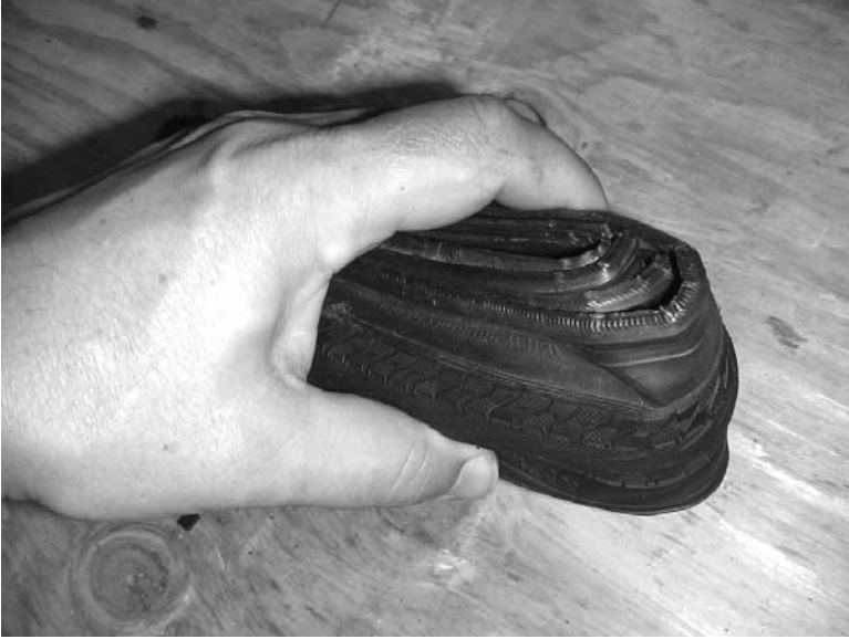
Folding spare tires are small and can be a life saver in remote areas.
